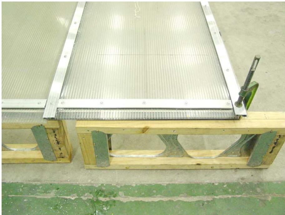
**Figure 1. View of 10mm sheets on the test frame**
