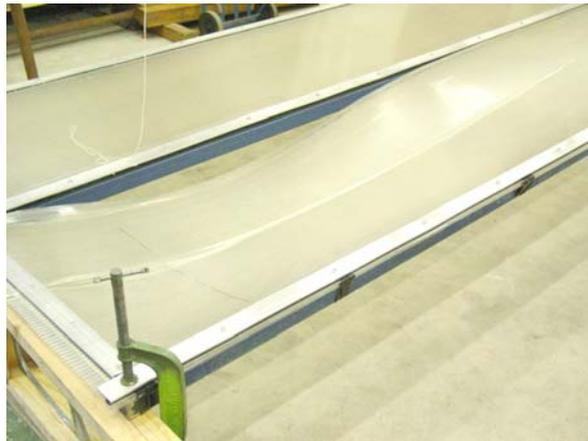
**Figure 4. Damage to 10mm aged sheet after removal of the test bag**
