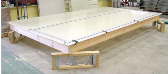
View of New 16mm sheet prior to test, note the short section to finish the end detail
