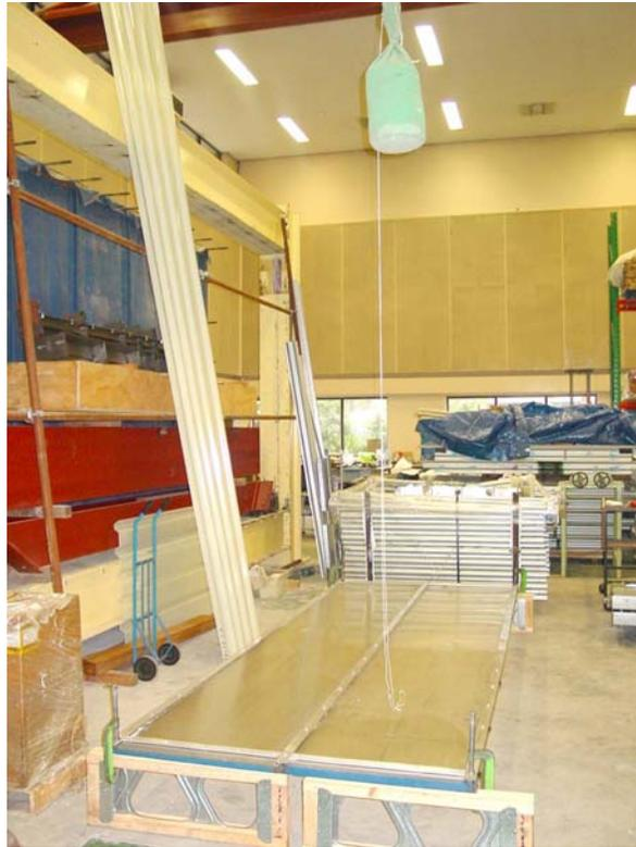
**Figure 3. View of 10mm test specimen prior to dropping the bag**
